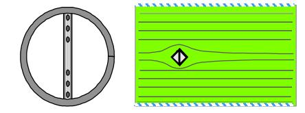
Low blockage of the Annubar® reduces permanent pressure drop!
